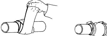
4. Wrap the inner tube as tightly as possible on the hose.
