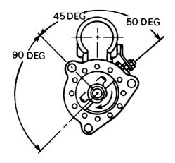
FIGURE 8-1-B. Pinion housing position for LD-465-1 and LD-465-1C, and LDT-465-1C engine applications.
