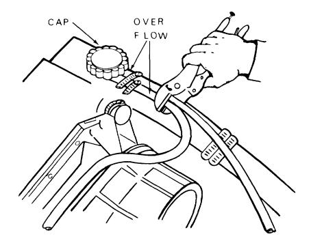
7. Plug overflow lines on surge tank coolant systems if so equipped.
