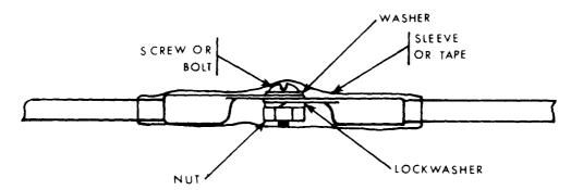
4. Bolt the terminal lugs together using short bolt with nut.
