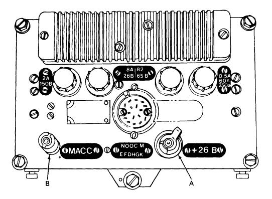
6. Jumper the red and the white wires to the positive side of the Soviet power supply (Point A). Use a jumper cable of at least 12-gauge wire.
