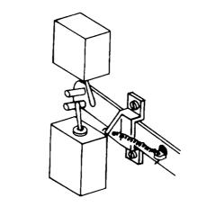
13. Turn the POWER switch to LOW position. Both of the circuit breaker levers should remain in the ON position.
