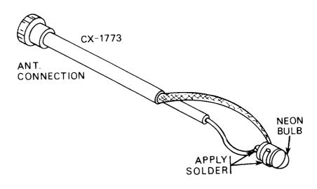
a. An RF transmitter output tester can be made from a neon light bulb and a piece of CG-1773 RF cable. Solder the bulb to the cable as shown in the illustration. Connect the cable to the ANT connection on the front of the radio. When the radio is keyed, the bulb will glow if RF power is present at the antenna connection (this does not verify transmitter frequency accuracy).
