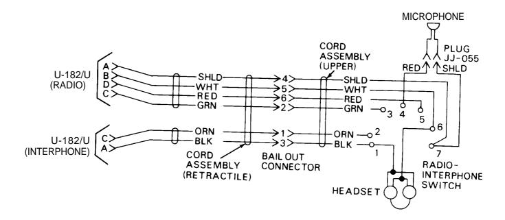
2. Connect four jumper wires, 12 feet long, to the white, black, red, and shield wire connections on the CVC helmet switch.
