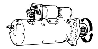
FIGURE 8-1-A. Pinion housing position for LDS-465-1 and LDS-465-1A engine applications.
