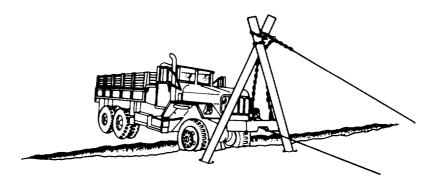
2. Lash the poles together at the top with a figure-eight or girth hitch as shown below.
