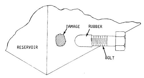
3. Insert slivers of wood if necessary to help ensure a better seal.
