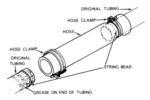
Option 2: Replacement of Long Damaged Tube Section.
