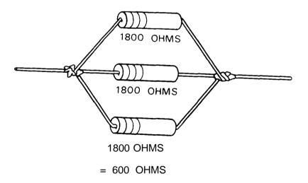
When the resistors are hooked in parallel, the resistance is reduced by the number of equal-value resistors in parallel.
