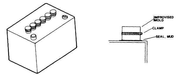
6. Melt approximately 6 oz of lead or solder in a metal can or cup and pour it into the improvised mold.
