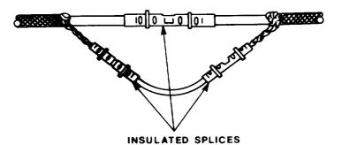
3. Use two splice connectors to add a short length of insulated wire as an extension to complete the shield connection.
