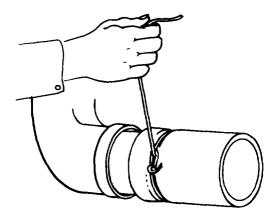
3. Press the loop tightly against the hose and pull the wire through the loop as tight as possible. Bend the wire back on itself, crimping it, so that the wrap will be tight and secure.
