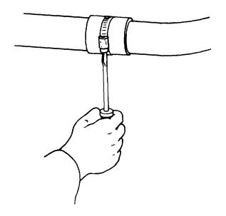
4. Wrap a nonporous material (raincoat, rubber mat) over the leak.
