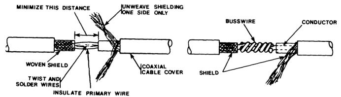
6. Lay the unwoven shielding over the insul ated splice and make contact with the woven shield on the other side. Distribute the unwoven shielding carefully around the diameter of the wire and solder or wrap with busswire.
