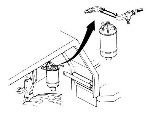
3. If a coupling is not available, cut the fittings off the fuel lines.
