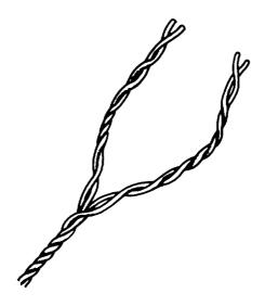
2. Bend the sets of strands into the desired loop, crossing over with one set in the same manner you would make a simple overhand knot. The two sets of strands will lock together.
