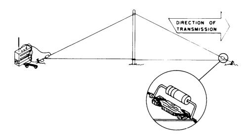
17. Connect a 600-ohm carbon resistor across the insulator on the transmission end of the antenna. Refer to paragraph 15-7 for construction of a 600-ohm resistor.
