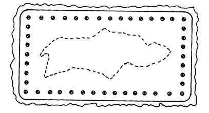
6. Dri11 holes in plate and tank approximately 1 inch apart. Apply sealer to the patch and rivet or screw the plate to the fuel tank.
