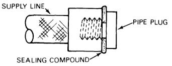
Option 3: High-Pressure Line Repair with a Cap. Procedural Steps:
