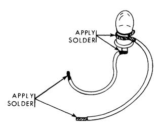
2. Making an ohmmeter (continuity tester).
