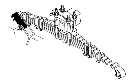
4. Weld the broken leaf springs with I/4-inch passes. A11ow each pass to cool. Keep alternating the welding process until all broken springs are welded.
