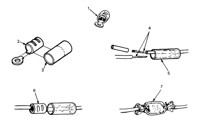
3. Cut insulating sleeve 1 inch longer than the barrel.
