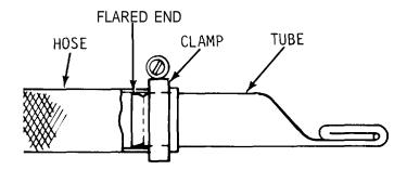
3. Flare other end of tubing, if possible, and remove burrs. Apply light coat of sealing compound around flared end of tube.
