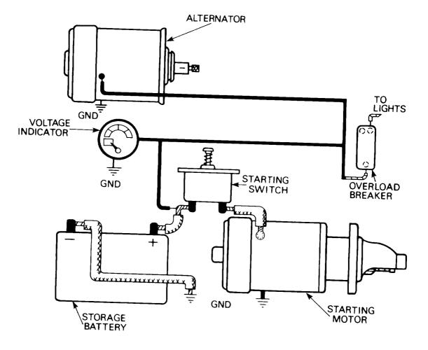
FIGURE 8-1. Basic vehicle electrical system.
