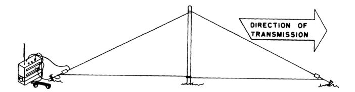
3. Move your vehicle approximately 50 feet from the support. Keep the support in line with and between you and the desired station.
