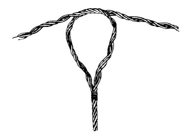
3. Start laying the strand sections alternately back into the rope grooves, continuing until sections are laid as deep into the throat as possible, allowing the six strands and core to project past the throat of the loop.
