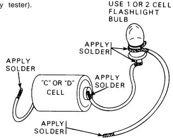
3. Making an RF Transmitter Output Tester.
