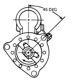
FIGURE 8-I-C. Pinion housing position for LD-465-2 engine applications.
