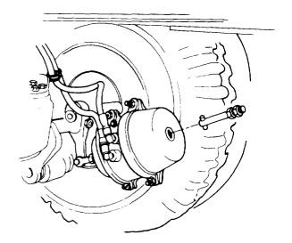
1. Use a caging bolt tool and turn in a direction that will retract the pushrod and compress the power spring in the brake chamber.
