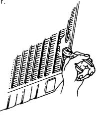
2. Inspect the radiator to pinpoint the leak.
